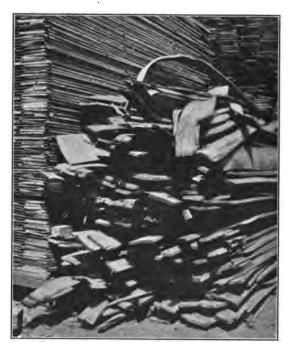
Fig. 85.—Partially rotted hardwood boards piled against a lumber stack. Infection will spread by contact to the sound lumber.
